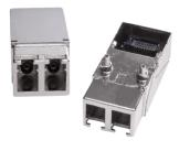
Moog Stiletto series optical fiber transceivers consist of 10 Gbps optoelectronic transmitter and receiver functions integrated into a pluggable Duplex LC compliant connector. The optical harsh environment transmitters are 850 nm VCSEL lasers. The transmitter input lines are driven with differential CML signals applied to the transmitter (TX+ and TX-) lines. Dual loop, temperature compensated, VCSEL drivers convert the transmitter input signals to suitable VCSEL bias and modulation currents.
