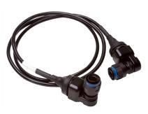
The electrical D38999 size 11-35 connector provides a rugged electrical interface that does not require cleaning or maintenance in order to perform in harsh environments. Signal conversion is done in the back shell of the electrical connector. The multimode or single mode optical fiber cable supports applications where copper cable link distance, bandwidth, weight or bulk make the use of twisted pair, twinax or quadrax copper conductors unacceptable.
